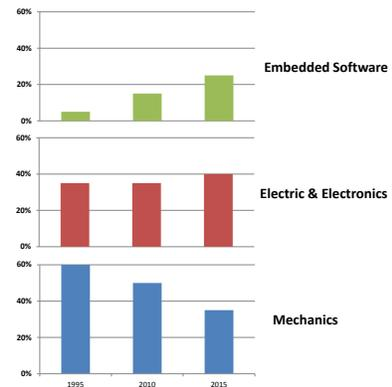
Figure 1: Percentage of domains in vehicle development (Source: A.T.Kearney Embedded Svstems Studv 2010)
